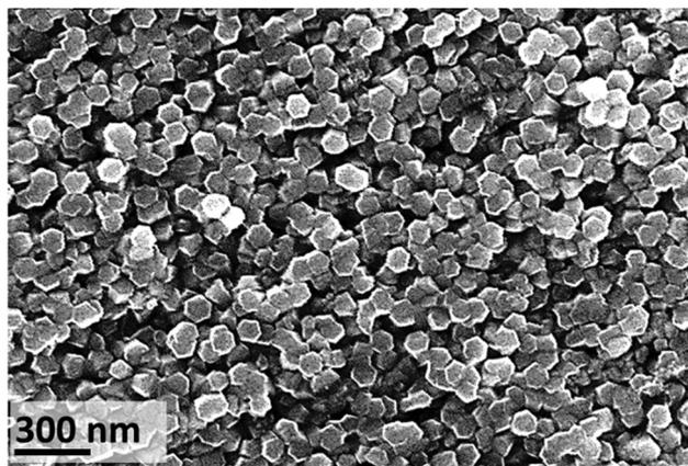
Fig. 7 SEM image of zinc substrate after exposure to [C<sub>4</sub>C<sub>1</sub>im]Cl (IL-1,  $X_{\text{H}_2\text{O}} = 0.75$  solution,  $20 \pm 1$  °C) for 26 d, showing the top of hexagonal nanorods (average size  $150 \pm 30$  nm,  $n = 278$ ).
