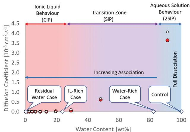
Fig. 1 Structural and diffusion properties of  $[C_4C_{1im}]Cl/water$  mixtures as a function of water concentration. Diffusion data calculated from MD simulations at 350 K.<sup>35</sup> White circle (○) chloride, red circle (●)  $[C_4C_{1im}]^+$ .
