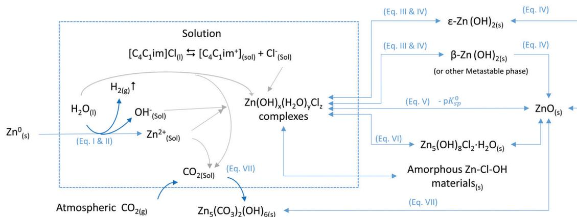
Fig. 9 General conversion paths of metallic zinc into ZnO in [C<sub>4</sub>C<sub>1</sub>im]Cl/water systems. Equations in the scheme are not balanced. Equations are given in the text. The predominant path and species formed will depend on the temperature and water content.
