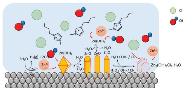
Fig. 5 Cartoon of Zn-based micro/nano particles in [C<sub>4</sub>C<sub>1</sub>im]Cl at high water content. At this water content, chloride anions can diffuse freely to react with Zn cations to form Zn–Cl compounds.
