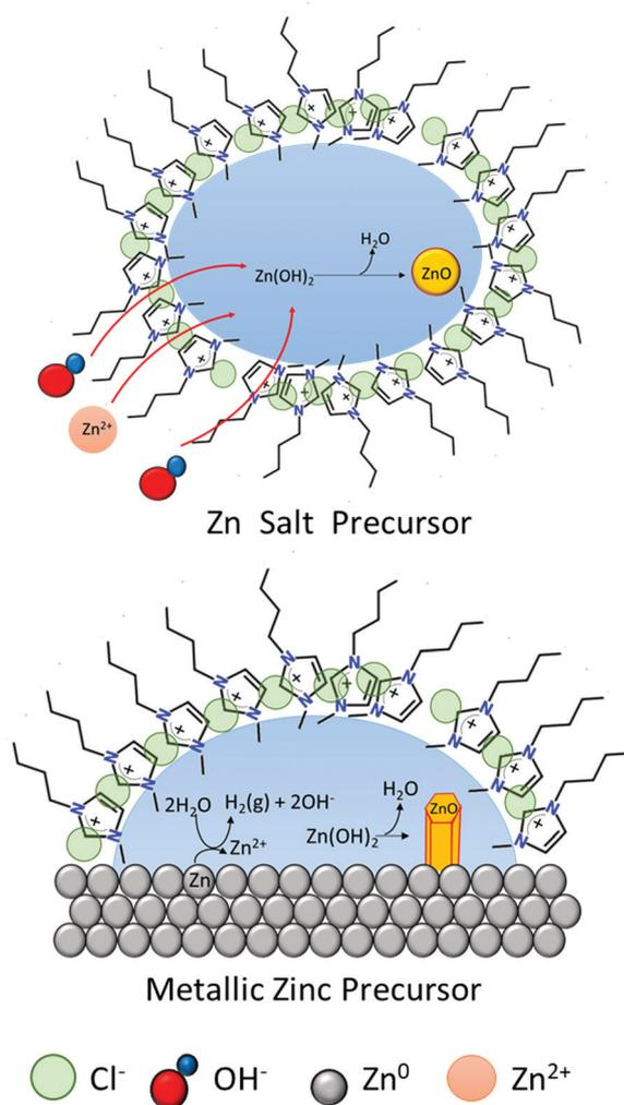
Fig. 8 Schematic of ZnO formation in [C<sub>4</sub>C<sub>1</sub>im]Cl at low water content. Left: Zn salts as precursors.<sup>40</sup> Right: Metallic zinc as precursor.
