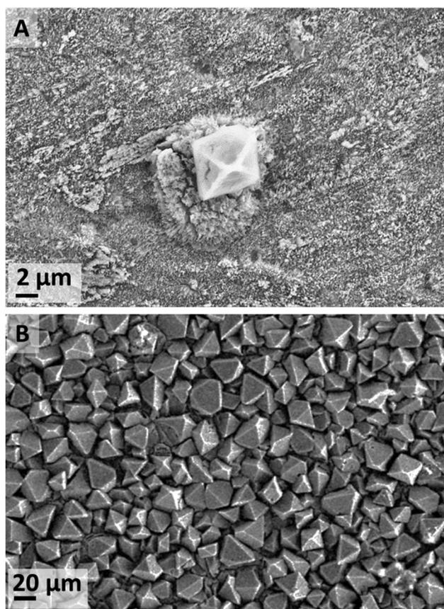
Fig. 3 SEM image showing zinc surface exposed to  $[C_4C_{1im}]Cl$  (IL-1,  $X_{H_2O} = 0.98$  solution at  $20 \pm 1$  °C). (A) Single octahedron  $Zn(OH)_2$  particle after 18 d exposure (approximate length of  $7.9 \pm 0.6$  μm). (B) Multiple  $Zn(OH)_2$  crystals after 44 d exposure with a mean length of  $21 \pm 6$  μm ( $n = 84$ ).
