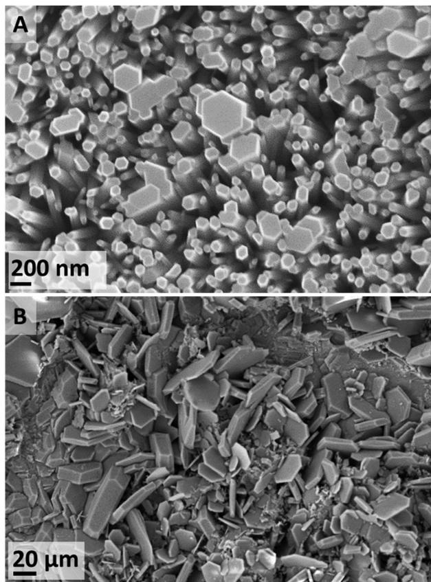
Fig. 4 Magnified zinc surface exposed to [C<sub>4</sub>C<sub>1</sub>im]Cl (IL-1, X<sub>H<sub>2</sub>O</sub> = 0.98 solution at 70 ± 1 °C). (A) ZnO nanorods after 4 d exposure (magnification 134.17k $\times$ ) (average size 90 ± 40 nm,  $n$  = 361). (B) ZHC plate-like crystals after 15 d exposure (magnification 1.44k $\times$ ). Estimated thickness 2.5 ± 1.5  $\mu$ m ( $n$  = 85), diameter 19 ± 8  $\mu$ m ( $n$  = 85).
