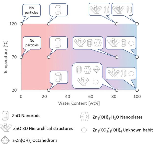
Fig. 2 Graphical summary of Zn-based materials, obtained by direct oxidation of metallic zinc in  $[C_4C_{1im}]Cl$  solutions, as a function of experimental conditions. Further details are provided in Tables S1 and S2 in ESI<sup>†</sup>.
