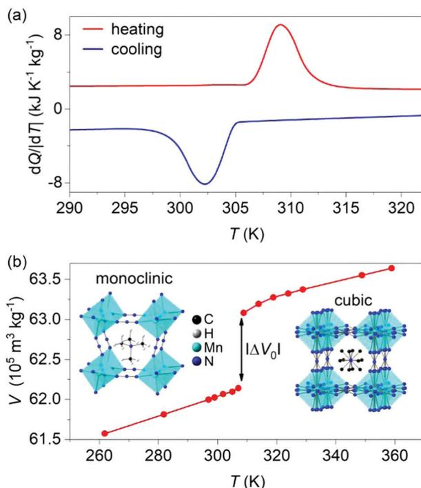
**Fig. 1** (a) Heat flow  $dQ/dT$  as a function of temperature, at atmospheric pressure. (b) Specific volume as a function of temperature, at atmospheric pressure, measured on heating via variable-temperature synchrotron powder X-ray diffraction. Left inset: pseudo-cubic representation of the low-temperature monoclinic phase; right inset: pseudo-cubic representation of the high-temperature cubic phase. H atoms in the high temperature phase are omitted for clarity of visualisation.
