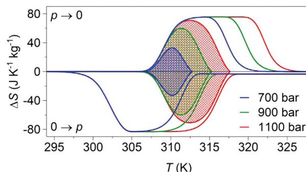
**Fig. 3** Pressure-driven isothermal changes in entropy on applying ( $0 \rightarrow p$ ) and removing ( $p \rightarrow 0$ ) selected hydrostatic pressures. Data shaded using different colours represent the reversible<sup>18</sup> barocaloric response at different pressures.
