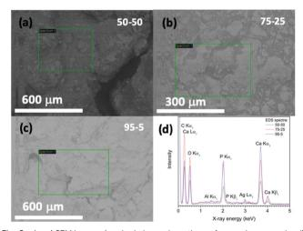
Fig. 8 (a–c) SEM images (marked places show the surface regions examined) and (d) EDS spectra of acrylate–gelatin–cHAP composite scaffolds.
