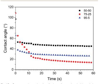
Fig. 12 Contact angles vs. time (sessile drop of water tinted with methylene blue dye) on acrylate-gelatin-cHAP composite scaffolds (values of the first measurement are presented)
