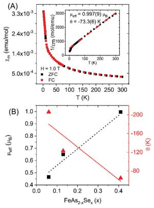
Fig. 4 (A)  $\chi_m vs. T$  for FeAs<sub>1.50</sub>Se<sub>0.50</sub> single crystals (FC is shown in red, ZFC is shown in black). The inlay shows  $1/\chi_m$  vs. T with the Curie-Weiss fit from 100 K to 300 K. (B) Calculated values of  $\mu_{\rm eff}$  and  $\theta$  (A) vs. Se fraction  $(x = 0.06 \text{ and } 0.13 \text{ are from literature}).^{10}$
