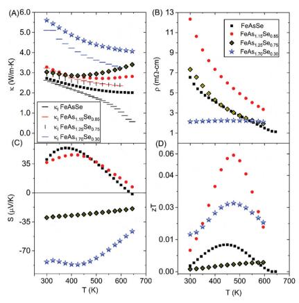
Fig. 6 Total thermal conductivity ( $\kappa_{lol}$ ) given as symbols and lattice thermal conductivity ( $\kappa_{l}$ ) provided as dashes (A), resistivity (B), Seebeck coefficient (C), and zT (D) measured on sintered polycrystalline pellets of FeAs<sub>2-x</sub>Se<sub>x</sub> (x = 0.3, 0.75, 0.85, 1.0).
