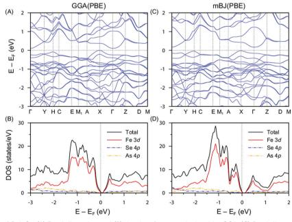
Fig. 7 Electronic structure of FeAsSe. (A) Band dispersion and (B) density of states calculated by GGA. (C) Band dispersion and (D) density of states calculated by mBJ.
