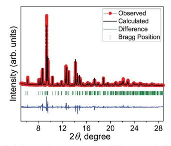
Fig. 2 Rietveld refinement of synchrotron PXRD pattern of FeAsSe (arsenopyrite structure type, space group  $P2_1/c$ ). Color code: red dots = observed pattern, black line = calculated pattern, green bar = Bragg position, blue line = difference between observed and calculated patterns.
