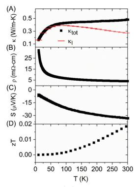
Fig. 5 Total thermal conductivity  $(\kappa_{\rm tot})$  and lattice thermal conductivity  $(\kappa_{\rm l})$  (A), resistivity (B), Seebeck coefficient (C), and zT (D) measured on a FeAs<sub>1.50</sub>Se<sub>0.50</sub> single crystal.
