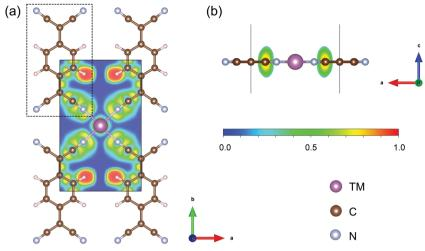
Fig. 1 (a) Top and (b) side view of the optimized structure of Sc-TCNQ and the corresponding electron localized function contour map. Sc, C, N, and H atoms are represented in purple, brown, cyan, and pale pink, respectively. Black solid line denotes the cell boundary of Sc-TCNQ, and the dashed line denotes the TCNQ molecule. Isodensity values for ELF map are shown below Fig. 1b.
