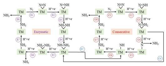
Fig. 2 Schematic illustration of enzymatic, consecutive, and their mixed mechanism for the NRR on TM-TCNQ. TM denotes the transition metal atom (active site) in the figures.
