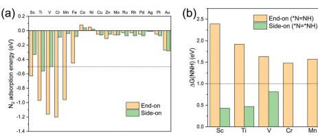
Fig. 3 The two-step screening strategy for TM-TCNQ electrocatalysts for the NRR. (a) Calculated  $N_2$  adsorption energy for both end-on and side-on configurations on TM-TCNQ (TM = Sc-Zn, Mo, Ru-Pd, Ag, Pt, and Au), and (b) Gibbs free energy change values  $\Delta G(NNH)$  of \*N  $\equiv$  N + (H<sup>+</sup> + e<sup>-</sup>)  $\rightarrow$  \*N=NH for Sc-, Ti-, V-, Cr-, Mn-, Fe-TCNQ, and \*N  $\equiv$  N\* + (H<sup>+</sup> + e<sup>-</sup>)  $\rightarrow$  \*N=NH\* for Sc-, Ti-, V-TCNQ.
