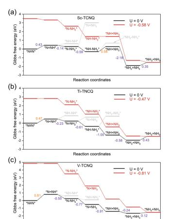
**Fig. 5** Gibbs free energy diagram for the NRR through the enzymatic/consecutive/mixed mechanism on (a) Sc-TCNQ, (b) Ti-TCNQ, and (c) V-TCNQ at zero and applied potential U. For U=0, reaction pathways and intermediates with unfavorable Gibbs free energy change are marked in grey, and the Gibbs free energy changes for each step are marked and shown in eV (value marked in orange color denotes the potential limiting step).
