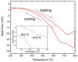
Fig. 4 DSC analysis in argon for microwave-hydrothermal-synthesized  $Sn_{1-\delta}S$  in two consecutive heating and cooling cycles.
