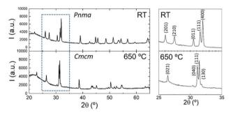
Fig. 5 X-ray powder diffraction pattern of  $Sn_{1-\delta}S$  at room temperature and at 650 °C, showing the structural transition from the Pnma (room temperature) to the Cmcm space group at high temperatures. A magnification of the area enclosed by the dashed line is shown in the left part of the figure, including the Miller indices for the reflections.
