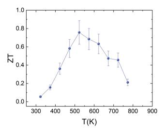
Fig. 11 Temperature dependence of the figure of merit (ZT) for  $Sn_{1-\delta}S$ synthesized using the microwave-hydrothermal method
