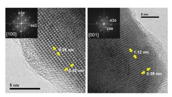
Fig. 3 Experimental HRTEM micrographs along the [100] and [001] zone axes. FFT images are shown in the insets.
