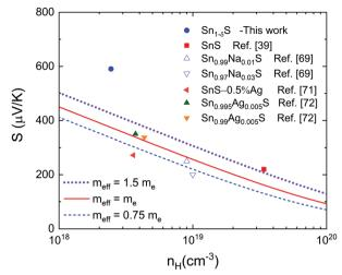
Fig. 9 Pisarenko lines for different effective masses at room temperature showing the single parabolic band model prediction for the Seebeck coefficient *versus* carrier concentration  $(n_{\rm H})$  in comparison with our measurement and literature data.
