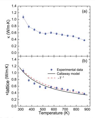
Fig. 10 Temperature dependence of the (a) total thermal conductivity and (b) lattice thermal conductivity of microwave-synthesized  $\mathrm{Sn}_{1-\delta}\mathrm{S}$ . The black solid line represents the data calculated using the Callaway model, <sup>76</sup> while the dotted line shows the  $\sim \mathcal{T}^{-1}$  fit.
