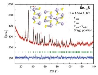
Fig. 2 Rietveld refinement from the powder neutron diffraction data of microwave-synthesized  $\mathrm{Sn}_{1-\delta}\mathrm{S}$ : observed (red crosses), calculated (black line) and difference (blue line) profiles. The allowed Bragg positions are shown as green vertical marks. The crystalline structure obtained from the refined data is shown in the upper part of the figure (Sn atoms are represented in purple and S atoms in yellow).
