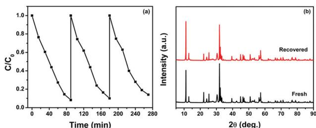
**Fig. 11** (a) Photocatalytic activity of the BiOBr/g-C<sub>3</sub>N<sub>4</sub> composite towards CR dye degradation for three cycles and (b) PXRD patterns of fresh and recovered catalysts.
