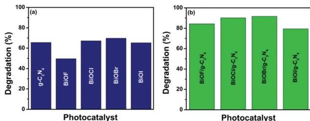
Fig. 9 Photocatalytic activity plots presenting the percentage of degradation of CR dye under sunlight irradiation for a stipulated time of 90 min using (a) bare BiOX and g-C<sub>3</sub>N<sub>4</sub> as catalysts and (b) different BiOX/g-C<sub>3</sub>N<sub>4</sub> composites as catalysts.
