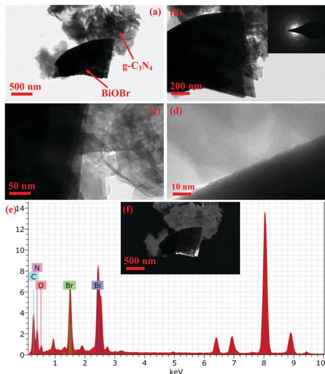
Fig. 6 (a–c) TEM images along with the diffraction pattern in the inset, (d) HRTEM image, (e) EDAX spectra and (f) dark field TEM image of the BiOBr/g-C<sub>3</sub>N<sub>4</sub> composite.
