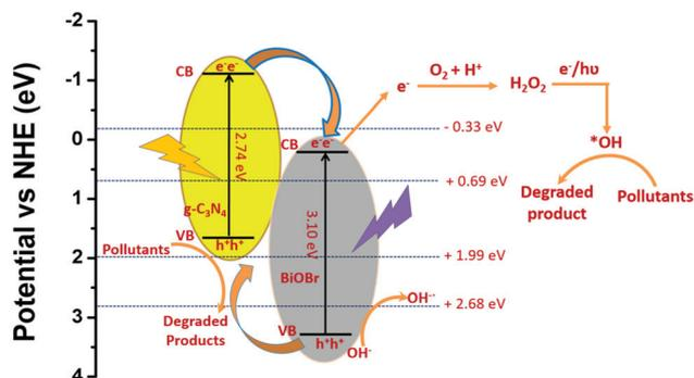
**Scheme 3** Plausible mechanism of degradation of CR under sunlight irradiation over the BiOBr/g-C<sub>3</sub>N<sub>4</sub> composite.
