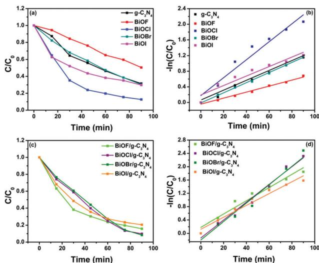
Fig. 10 Kinetic curves obtained by applying a pseudo first order kinetic model for the photo-degradation of CR dye using (a and b) different bare BiOX and g-C<sub>3</sub>N<sub>4</sub> and (c and d) different BiOX/g-C<sub>3</sub>N<sub>4</sub> composites.
