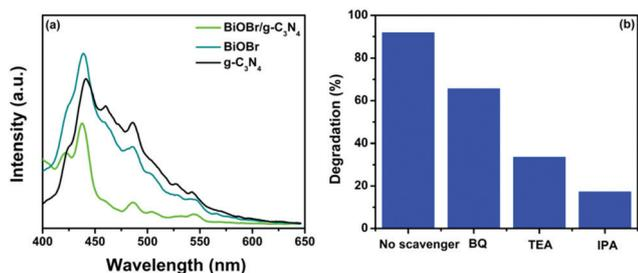
**Fig. 12** (a) PL spectra of g-C<sub>3</sub>N<sub>4</sub>, BiOBr and the BiOBr/g-C<sub>3</sub>N<sub>4</sub> composite and (b) effect of scavengers on the photocatalytic activity of the BiOBr/g-C<sub>3</sub>N<sub>4</sub> composite towards CR degradation under sunlight irradiation.
