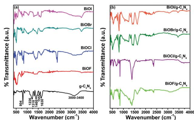
Fig. 2 FTIR spectra of (a)  $g\text{-C}_3\text{N}_4$ ,  $\text{BiOX}$  ( $X = \text{F}, \text{Cl}, \text{Br}$  and  $\text{I}$ ) and (b)  $\text{BiOX}/g\text{-C}_3\text{N}_4$  composites.
