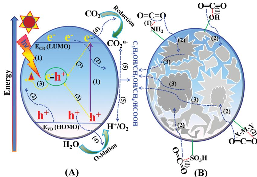
**Scheme 12** Basic mechanism of the photocatalytic process: (A) optoelectronic steps and (B) physicochemical steps involved in the CO<sub>2</sub> reduction reaction.
