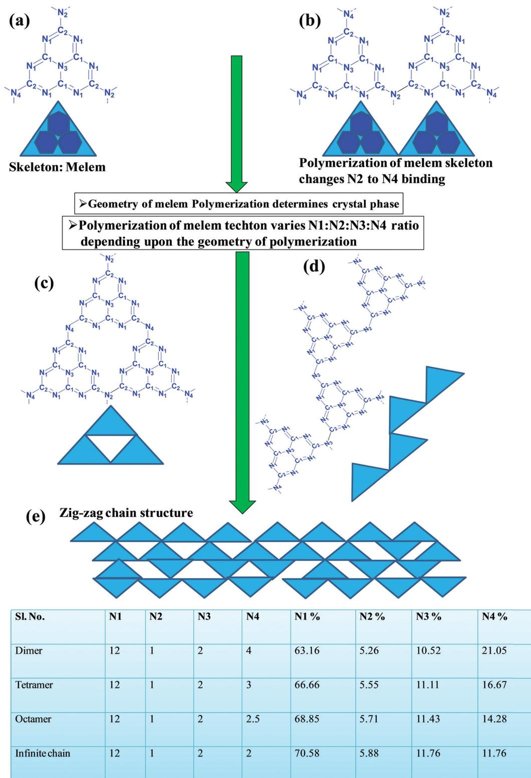
Scheme 4 Evolution of different geometry and N types present in  $C_3N_4$  based on the variation of the linkages of melem units.<sup>53</sup>
