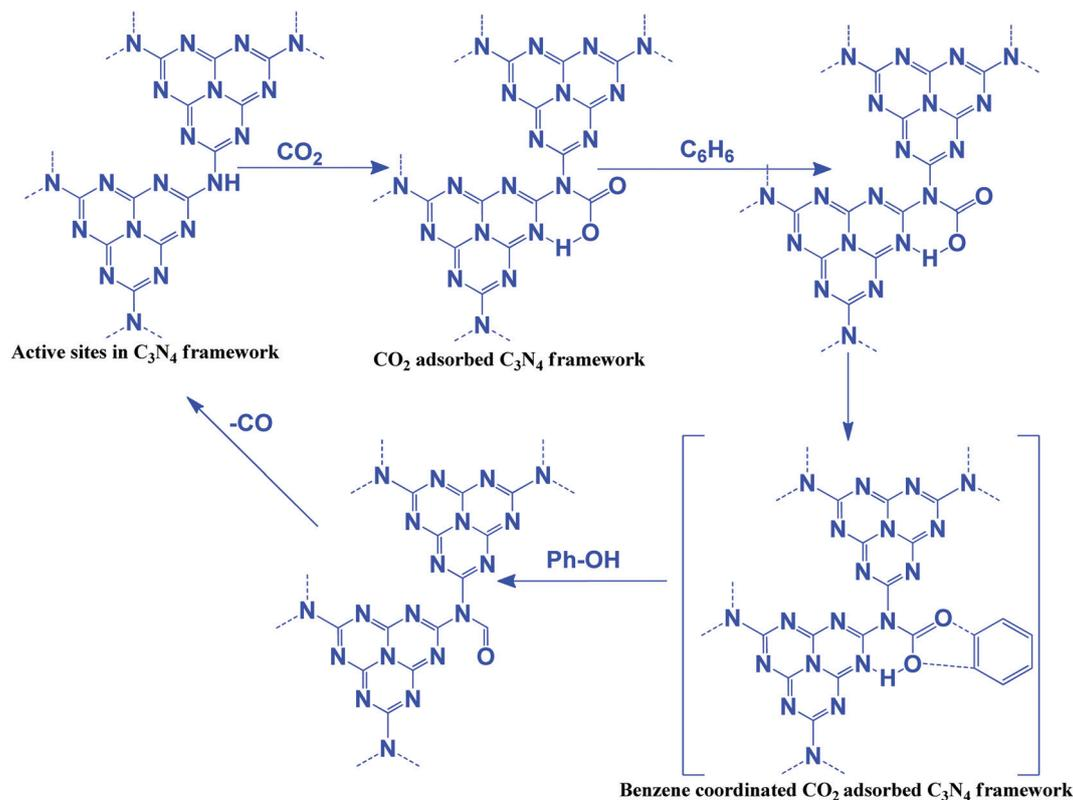
Scheme 10 Oxidation of benzene to phenol using CO<sub>2</sub> as an oxidant and g-C<sub>3</sub>N<sub>4</sub> as a catalyst.
