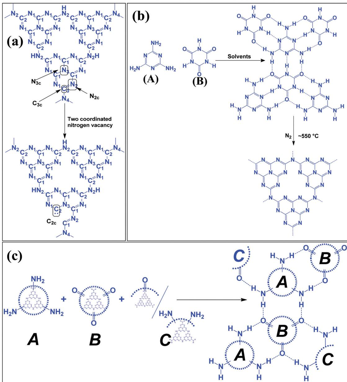
Scheme 8 Supramolecular assembly of precursors leading to formation of mesoporous g-C<sub>3</sub>N<sub>4</sub>.
