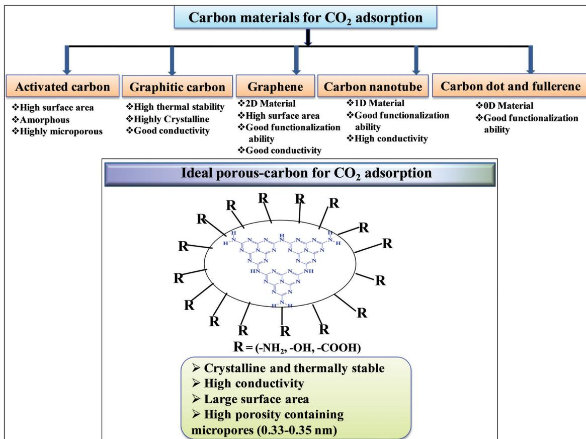
Scheme 2 Porous carbon materials for CO<sub>2</sub> adsorption.
