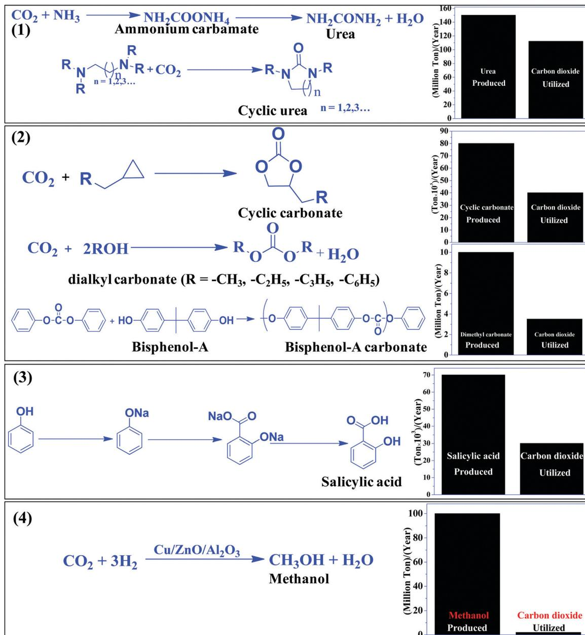
Scheme 1 CO<sub>2</sub> based commercial processes and amount of CO<sub>2</sub> utilized vs. product formed in the given process.
