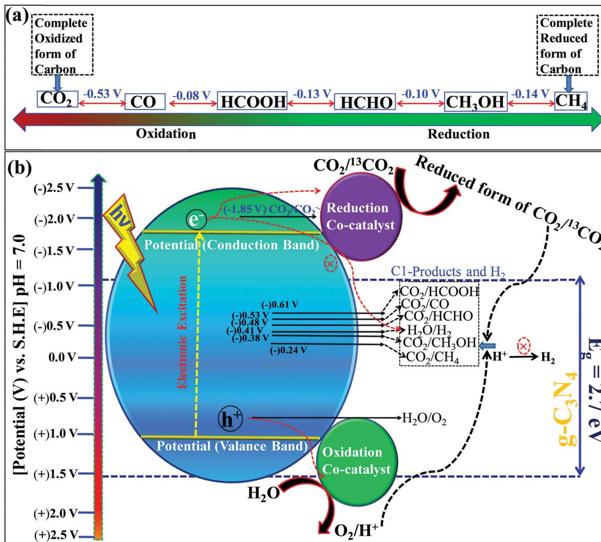
Scheme 13 (a) The different states of carbon with the potential difference, and (b) photocatalytic CO<sub>2</sub> reduction with respect to the standard redox potential of different products and band straddling.
