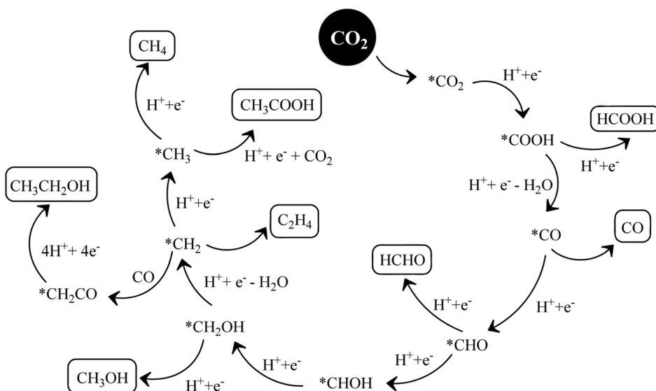
**Scheme 17** Various products formed due to multi-step processes during electrochemical CO<sub>2</sub> reduction.
