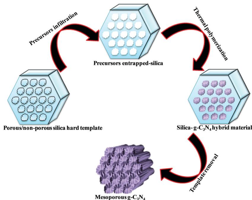
Scheme 7 Hard template mediated synthesis of mesoporous  $g\text{-C}_3\text{N}_4$ .
