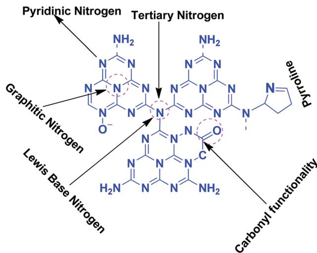
Scheme 5 Different types of N and O functionalities present in  $g\text{-C}_3\text{N}_4$ .
