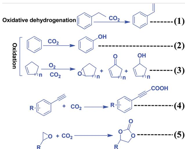
Scheme 9 Synthesis of organic compounds using CO<sub>2</sub> as a reactant or oxidant or promoter and C<sub>3</sub>N<sub>4</sub> as a catalyst.
