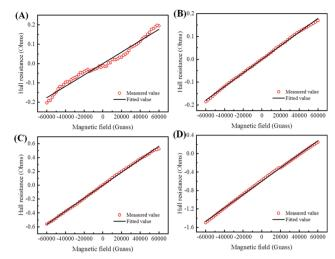
Fig. 5 The Hall resistance value as a function of magnetic field for the optimized Te NWs thin piece (A and C) and that synthesized with  $N_2H_4$ - $H_2O$  (B and D) before (A and B) and after (C and D) annealing at 350 °C for 3 h.
