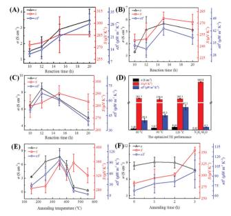
Fig. 3 Reaction condition-dependent TE performance of the Te NWs thin pieces, where the Te NWs were synthesized with glucose at 60  $^{\circ}$ C (A), 90  $^{\circ}$ C (B), 120  $^{\circ}$ C (C) for different times. A comparison of the optimized TE performance of the Te NWs thin pieces (D). The TE performance of the optimized Te NWs thin pieces as a function of annealing temperature (E) and time (F).
