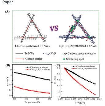
Fig. 4 Schematic illustration of the highly conductive Te NWs synthesized with glucose (A). The dependence of electrical conductivity on temperature (B) and analysis of the temperature-dependence of the electrical conductivity with the 1D VRH model (C) of the optimized Te NWs thin piece and that synthesized with  $N_2H_4$ : $H_2O$  before annealing.
