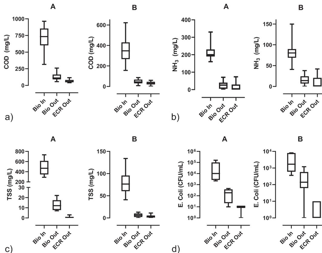
Fig. 4 Water quality parameters (a) COD, b)  $\text{NH}_3$ , c) TSS, and d) *E. Coli* before biological pretreatment (Bio In), after biological pretreatment (Bio Out), and after electrochemical disinfection (ECR out); lines in the boxes represent medians, the boxes are the 25th and 75th percentiles, and the error bars are the minimum and maximum values. For the numerical values and sample sizes ( $n$ ), see Table S5.†
