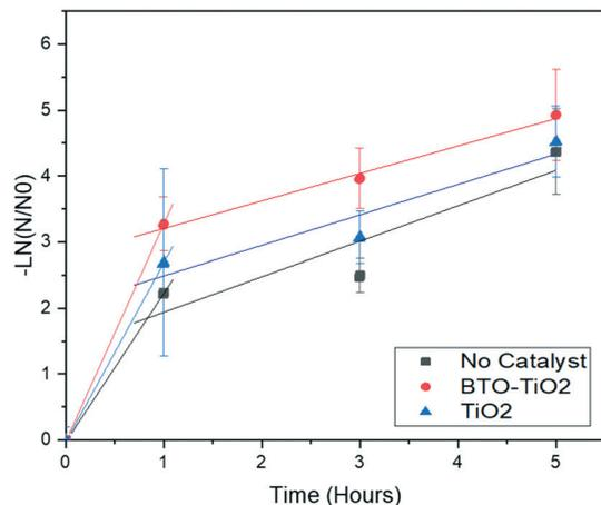
Fig. 6 Linearized rate of disinfection for W2B water, obtained by taking the negative natural log of the normalised colony counts, showing the difference in rates between  $t = 0$  to 1 hour and  $t = 1$  to 5 hours.
