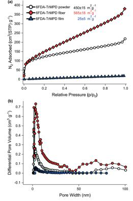
Fig. 4 a) Nitrogen adsorption isotherms measured at -196 °C up to 1 bar, b) NLDFT-derived pore size distributions of the 6FDA-TrMPD polymer powder, the nanofibrous mat and the film.
