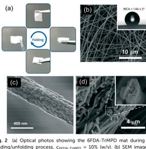
Fig. 2 (a) Optical photos showing the 6FDA-TrMPD mat during the folding/unfolding process,  $c_{\rm 6FDA-TrMPD}=10\%$  (w/v). (b) SEM image of the nanofibers and its water wettability showing hydrophobicity. (c) SEM image of a single nanofiber showing a wrinkled texture. (d) Cross-section image of the mat and fiber (inset).
