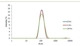
Fig. 2 Average DLS result for FITC RB nanosensors in pre-conditioned HH Combo medium over 24 h.
