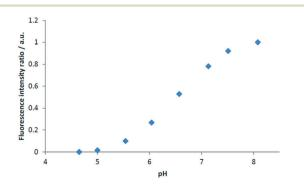
Fig. 4 FITC RB nanosensors calibration in HH Combo medium, normalised fluorescence intensity ratio of IFITC/IRB with varying pH.
