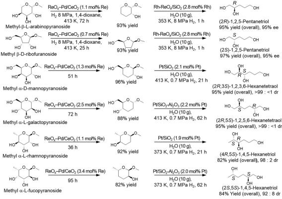
Scheme 30 Transformation of methyl glycosides to the corresponding chiral polyols by DODH, HG, hydrolysis and HG with ReO<sub>x</sub>-Pd/CeO<sub>2</sub> and hydrogenation catalysts. 37,39
