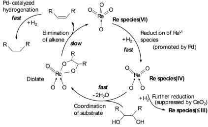
Scheme 29 Catalytic cycle of DODH and HG of polyols with  $ReO_x$ -Pd/CeO<sub>2</sub> catalyst.  $^{38}$
