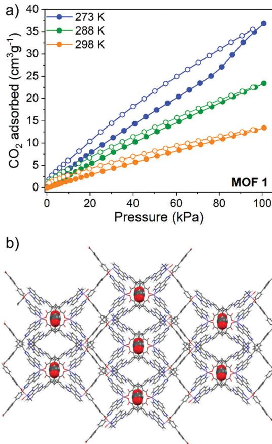
Fig. 2 (a) CO<sub>2</sub> adsorption (filled circles) and desorption (open circles) isotherms for **1** and (b) DFT-D3 optimization showing the preferential site of adsorption of CO<sub>2</sub> in **1**.
