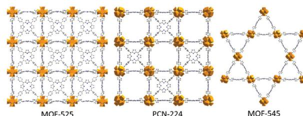
Fig. 1 The three porphyrinic  $Zr_6$ -TCCP-based MOFs encountered in this study. MOF-525 and PCN-224 exhibit cubic cavities, and PCN-224 being described as a MOF-525 with missing linkers. MOF-545 possesses hexagonal channels.
