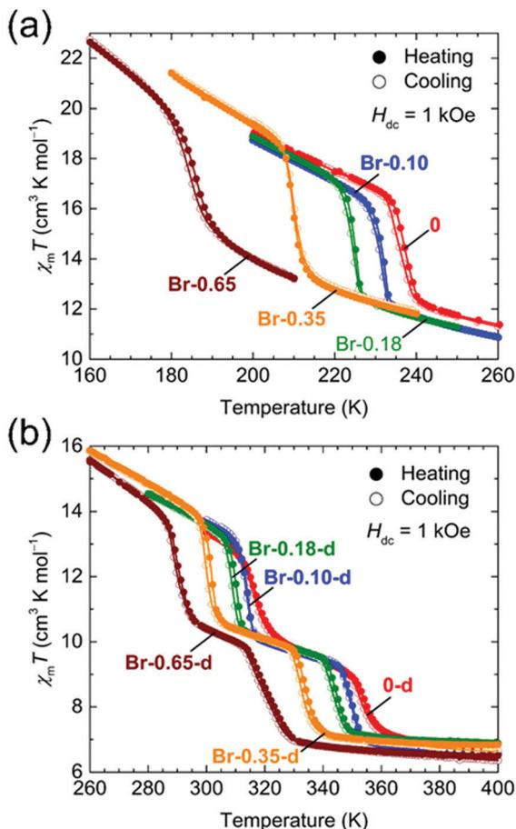
Fig. 2 Temperature dependence of  $\chi_m T$  for **Br-Y** (a) and **Br-Y-d** (b) measured at  $H_{dc} = 1$  kOe ( $\chi_m = M_m/H_{dc}$ ), where the narrow temperature ranges of 160–260 K and 260–400 K, respectively, were used.
