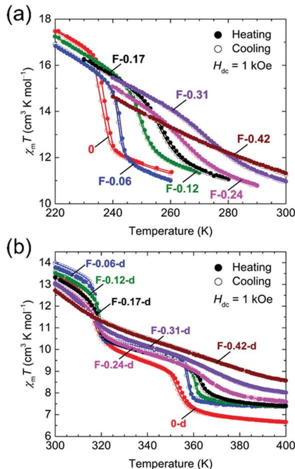
Fig. 3 Temperature dependence of  $\chi_m T$  for **F-Y** (a) and **F-Y-d** (b) measured at  $H_{dc} = 1$  kOe ( $\chi_m = M_m/H_{dc}$ ), where narrow temperature ranges of 220–300 K and 300–400 K, respectively, were used.
