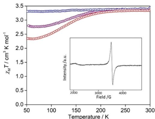
Fig. 5  $\chi_M T$  vs.  $T$  plot of  $[\text{FeL}_a(\text{py}_2\text{TTF})]_n$  (red) and doped with iodine for 2 days (purple) and 2 weeks (blue). Inset: EPR spectrum of  $[\text{FeL}_a(\text{py}_2\text{TTF})]_n$  infused with iodine for 2 weeks showing an oxidised TTF signal.
