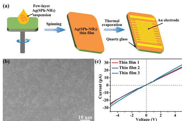
**Fig. 2** (a) Fabrication of Ag(SPh-NH<sub>2</sub>) thin film for gas sensing test. (b) Typical HR-SEM of the prepared Ag(SPh-NH<sub>2</sub>) thin films. (c) *I*-*V* curves of Ag(SPh-NH<sub>2</sub>) thin films.
