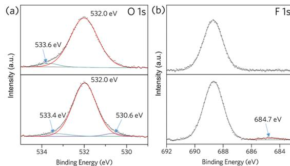
**Fig. 4** XPS spectra for (ZIF-62)<sub>0.2</sub>(6FDA-DAM)<sub>0.8</sub> (top) and (a<sub>g</sub>ZIF-62)<sub>0.2</sub>(6FDA-DAM)<sub>0.8</sub> (bottom), (a): O 1s, (b): F 1s.
