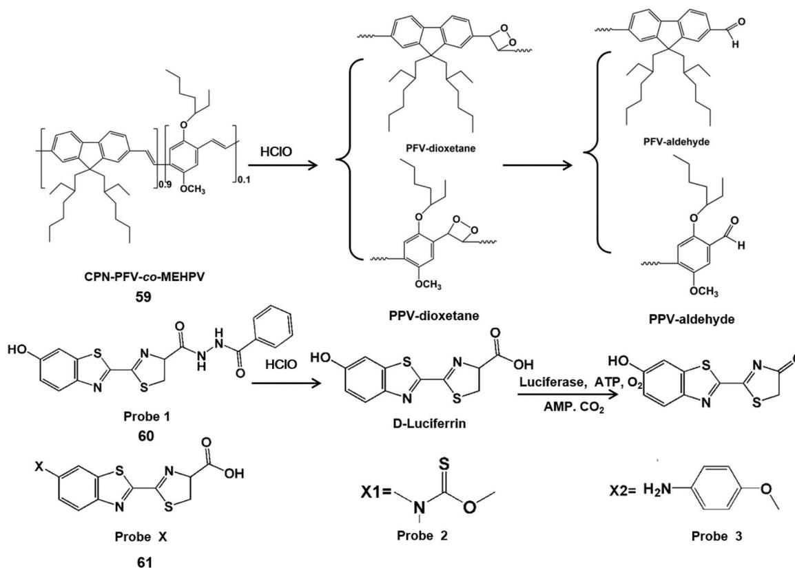
**Scheme 15** Structures and mechanism of chemiluminescent probes for HClO/CLO<sup>-</sup>. Reprinted with permission from ref. 128. Copyright 2018, American Chemical Society. Reprinted with permission from ref. 130. Copyright 2017, American Chemical Society. Reprinted with permission from ref. 131. Copyright 2018, Royal Society of Chemistry.
