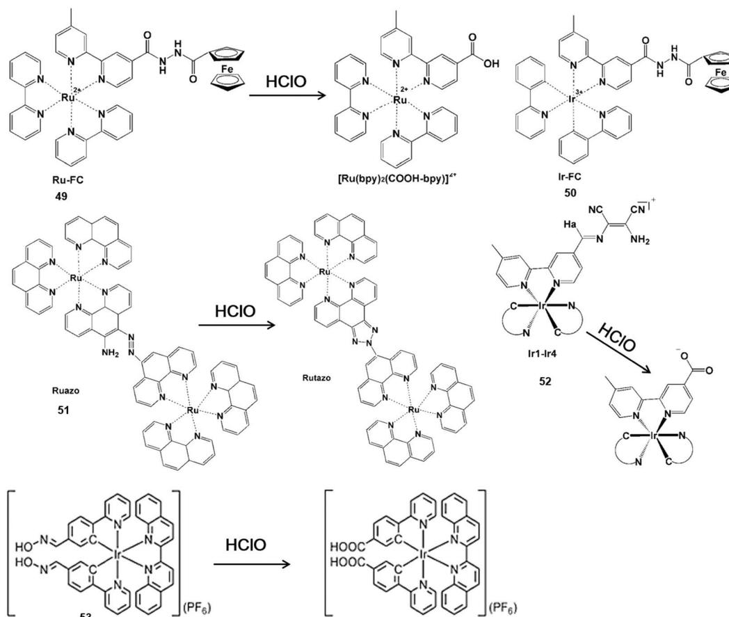
**Scheme 12** Structures and mechanisms of nitrogen-containing functional group probes for  $\text{HClO}/\text{ClO}^-$ . Reprinted with permission from ref. 109. Copyright 2015, Elsevier. Reprinted with permission from ref. 110. Copyright 2017, Elsevier. Reprinted with permission from ref. 111. Copyright 2016, Nature. Reprinted with permission from ref. 112. Copyright 2014, Royal Society of Chemistry. Reprinted with permission from ref. 113. Copyright 2015, Royal Society of Chemistry.
