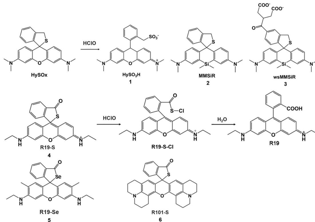
**Scheme 1** Structures and mechanisms of thioether ring-based probes for HClO/ClO<sup>-</sup>. Reprinted with permission from ref. 32. Copyright 2007, American Chemical Society. Reprinted with permission from ref. 33. Copyright 2011, American Chemical Society. Reprinted with permission from ref. 34. Copyright 2011, Royal Society of Chemistry.
