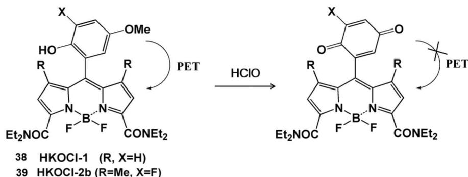
**Scheme 9** Structures and mechanism of the oxygen-containing nanoprobe in HClO/ClO<sup>-</sup>. Reprinted with permission from ref. 88. Copyright 2008, American Chemical Society. Reprinted with permission from ref. 89. Copyright 2014, American Chemical Society.
