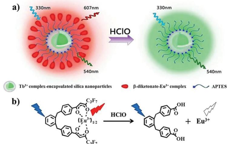
**Fig. 6** Design concept of a ratiometric luminescent probe based on crow-like dual-emissive silica nanoparticles modified by Tb<sup>3+</sup> and Eu<sup>3+</sup> complexes (a), and the luminescence quenching mechanism of a  $\beta$ -diketonate-Eu<sup>3+</sup> complex by HClO (b). Reprinted with permission from ref. 115. Copyright 2017, Royal Society of Chemistry.
