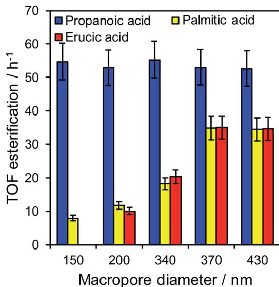
Fig. 3 Turnover frequencies for propanoic acid, palmitic acid, and erucic acid esterification over PrSO<sub>3</sub>H/MM-SBA-15 as a function of macropore diameter.
