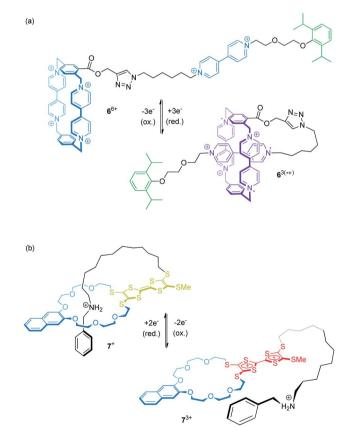
Fig. 7 Two examples for electrochemically controlled pseudo[1] rotaxanes which are convertible between a rope-like and a lasso-type conformation: (a) 66+ undergoes self-inclusion after reduction, whereas (b) 7<sup>+</sup> is preferentially threaded in the initial state and unthreads upon oxidation
