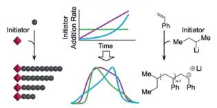
Fig. 3 Tailored shape and dispersity of the molecular weight distribution, produced *via* metered addition of *s*-BuLi to the anionic polymerisation of styrene. This figure is adapted from ref. 56 with permission from ACS publications.
