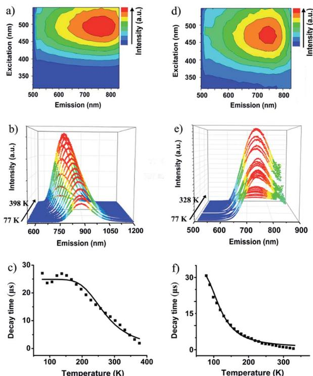
Fig. 3 3D Excitation-emission correlation spectra of (a) **1** and (d) **2** monitored in the solid state at 298 K. Temperature-dependent emission profiles of (b) **1** and (e) **2**. Temperature-dependent emission decay time of (c) **1** and (f) **2**; the solid line represents Boltzmann fitting to the experimental data.
