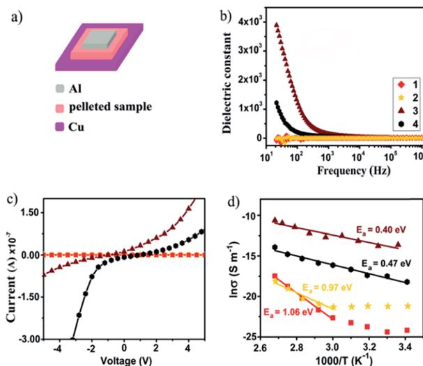
Fig. 6 (a) Fabrication of an electronic device for dielectric and electrical measurements. (b) Frequency-dependent dielectric constants of **1–4** recorded at room temperature. (c) Current–voltage curves recorded at room temperature. (d) Temperature-dependent electrical conductivity; straight lines represent Arrhenius fitting to the experimental data.
