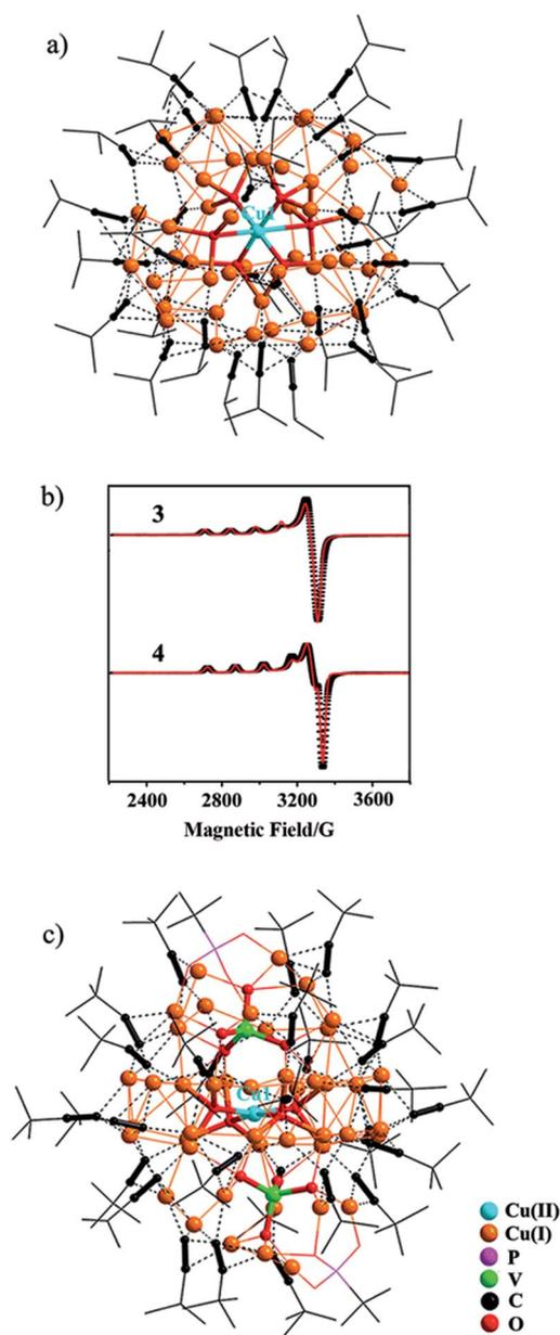
Fig. 2 Molecular structures of (a) **3**; (c) **4**. The Cu(II)–O–Cu(I) bonding interactions in **3** and **4** are highlighted as thicker bonds. (b) EPR spectra of **3** and **4**. Black and red lines represent the experimental and simulated EPR patterns, respectively.
