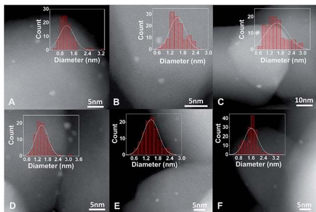
Fig. 2 HAADF-STEM and size distribution of Pt/TiO<sub>2</sub> catalysts. (A–C) and (D–F) are HAADF-STEM and size distribution of Pt/r-TiO<sub>2</sub>, Pt/h-TiO<sub>2</sub> and Pt/o-TiO<sub>2</sub> before and after reaction, respectively.
