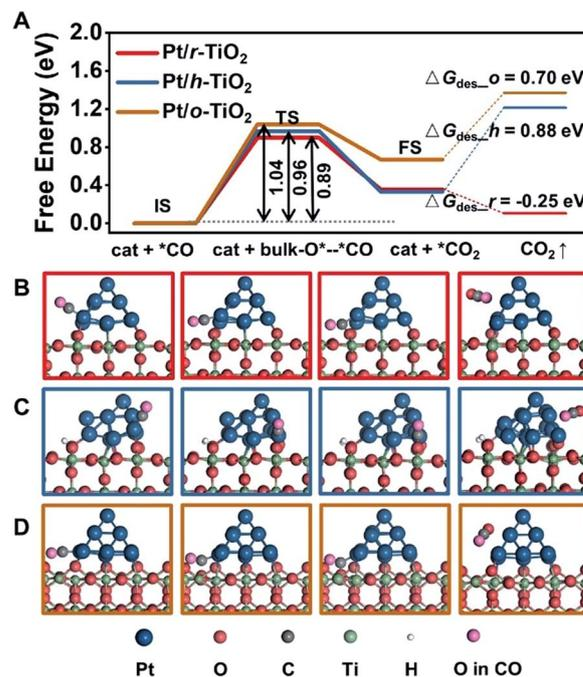
Fig. 4 Calculated CO oxidation over Pt/TiO<sub>2</sub> catalysts. (A) Free energy barriers for CO oxidation. (B–D) Models from left to right represent the initial state (IS), transition state (TS), final state (FS) and CO<sub>2</sub> desorption of CO oxidation on Pt/r-TiO<sub>2</sub>, Pt/h-TiO<sub>2</sub> and Pt/o-TiO<sub>2</sub>, respectively.
