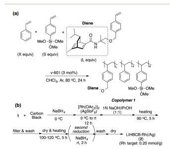
Scheme 2 Preparation of chiral polymer and catalyst.
