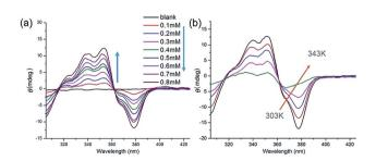
Fig. 3 (a) Concentration-dependent CD spectra of  $\bf 1$  in chloroform from 0.01 mM to 0.8 mM. (b) Temperature-varied CD spectra of  $\bf 1$  in chloroform from 303 K to 343 K.
