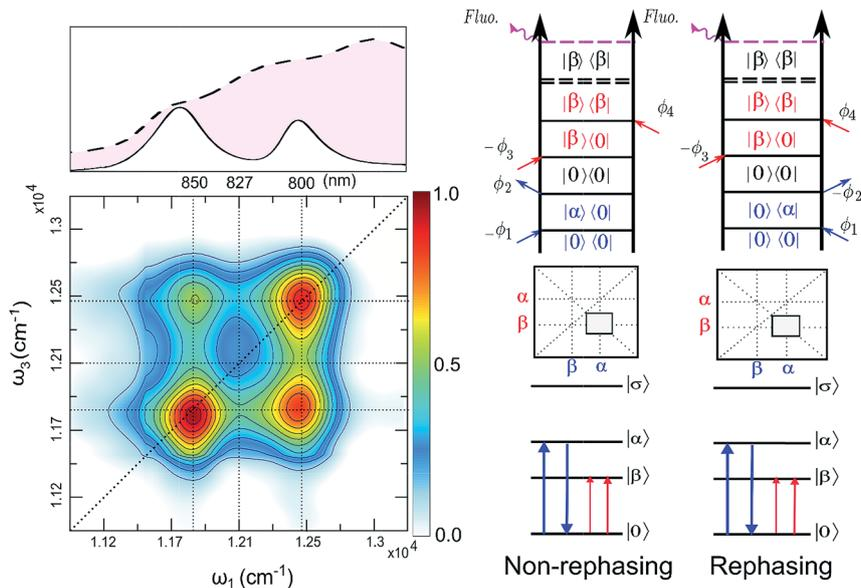
Fig. 4 (Left): Total (rephasing + nonrephasing) FD2D<sub>R+NR</sub> of LH2, at  $t_2 = 0$  fs, color scale normalized to one. Upper panel shows the absorption spectrum and the spectrum of the pulses (dashed) used in the experiment. (Right) Non-rephasing and rephasing GSB diagrams of the lower cross peak are shown.
