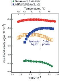
Fig. 8 (a) Ionic conductivity of Film-Cub<sub>bi</sub>(X) against the water content X. (b) Arrhenius plot of the ionic conductivity of Film-Cub<sub>bi</sub>(15.6) ( $\bullet$ ). As comparisons, that of N-MZI/HTf<sub>2</sub>N (1.0/1.0 by mol) containing 9.4 wt% of water ( $\blacksquare$ ), that of Film-Meso ( $\bullet$ ), and that of the GZI/HTf<sub>2</sub>N mixture containing 15.6 wt% of water ( $\square$ ) are also plotted.
