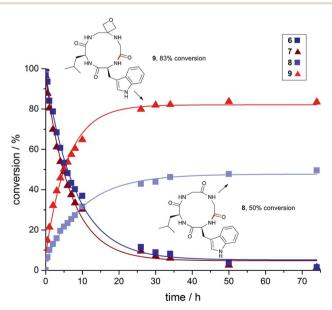
**Fig. 2** Impact of oxetane modification on macrocyclisation rates: Cyclisation of WLGG (**6**) and oxetane modified WLGOxG (**7**) monitored over 74 h using DEPBT (2 equiv.),  $^{\rm i}$ Pr<sub>2</sub>EtN (2 equiv.) in DMF (0.001 M), RT. Bond formed in macrocyclisation indicated in red; peptides were quantified by analytical HPLC by integration of the corresponding UV signal at 280 nm (see ESI†).
