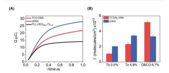
Fig. 4 (A) Example of CC curves measured for the gold electrodes modified with 0.25 mg mL $^{-1}$  of PLL–OEG(26.0)–Tz(4.9), 1  $\mu$ M TCO–DNA and cDNA in the presence of 50  $\mu$ M RuHex in 20 mM Tris buffer. (B) Surface coverage of Au electrode surfaces modified with PLL–OEG–Tz(0.5), PLL–OEG–Tz(4.9) and PLL–OEG–DBCO(6.7) and subsequently with TCO-DNA and N $_3$ -DNA, before and after hybridization with cDNA.
