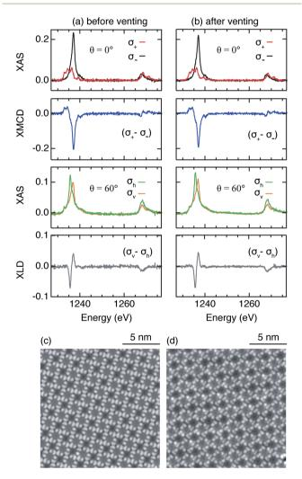
Fig. 4 XAS with circular polarizations, XMCD, XAS with linear polarizations, and XLD measured at the Tb  $M_{4.5}$  edge (a) before and (b) after exposure to ambient conditions for 1 hour (2.3 ML 2H-Pc/Ag(111) + 0.4 ML Tb;  $\mu_0 H = 100$  mT and 8.0 T for measurements with linear and circular polarizations, respectively, T=6 K). Representative STM images are shown in (c) and (d), respectively (2.7 ML 2H-Pc/Ag(111) + 0.8 ML Tb;  $V_t = -2.0 \text{ V}$ ,  $I_t = 20 \text{ pA}$ , T = 5 K).
