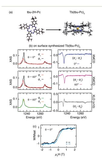
Fig. 5 (a) Schematic of tbu-2H-Pc and Tb(tbu-Pc)<sub>2</sub>. (b) XAS, XMCD, and XLD probed at the Tb M<sub>4.5</sub> edges and (c) magnetization curve probed at the Tb  $M_5$  edge (3.7 ML tbu-2H-Pc/Ag(111) + 0.8 ML Tb;  $\mu_0 H = 50$  mT and 6.8 T for measurements with linear and circular polarizations, respectively,  $\mu_0 \dot{H} = 2 \text{ T min}^{-1}$  for magnetization curves measurements, T = 3 K).
