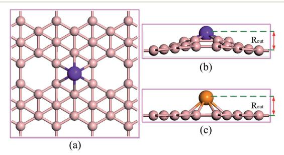
Fig. 1 Optimized geometric structure of the TM-B<sub> $\beta$ 12</sub> monolayers in the 3 × 3 computational supercell. (a) Top view, (b) and (c) side views. The pastel pink, orange and purple balls represent B, TM (TM = Sc, Cu and Zn) and TM (TM = Ti-Ni), respectively.  $R_{out}$  is the distance between the metal atom and the plane of the B $_{\beta$ 12</sub> sheet.
