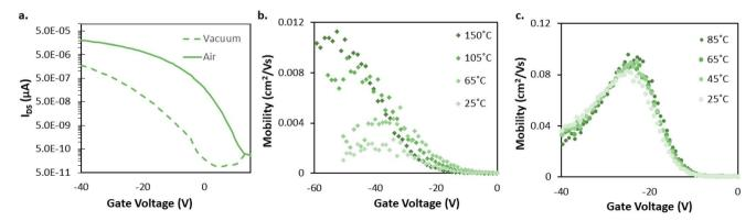
Fig. 2 Characterization of AlClPc OTFTs. (a) Transfer curves for AlClPc BGBC devices deposited at  $T = 140 \,^{\circ}$ C, and tested in air ( $V_{SD} = -50 \,^{\circ}$ V), and vacuum, at T = 25 °C.  $V_{GS}$  vs.  $\mu_{H}$  curves at temperatures ranging from 25 °C to 150 °C in vacuum (b) and temperatures from 25 °C to 85 °C in air (c).
