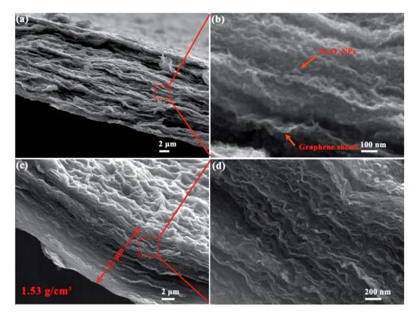
Fig. 1 Section view SEM images of the Fe<sub>3</sub>O<sub>4</sub>@rGO hybrid film (a and b) and the HWGF (c and d).
