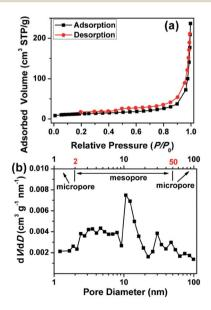
Fig. 3 (a)  $\mbox{N}_2$  adsorption isotherms and (b) pore size distributions calculated by BJH method of the HWGF.
