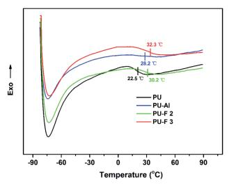
Fig. 6 DSC curves of PU, PU-Al (wt% = 1.86%), PU-F 2 (wt% = 0.71%) and PU-F 3 (wt% = 1.05%).
