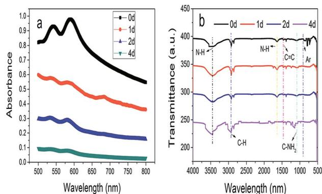
Fig. 9 Degradation products analysis of Disperse Red 3B by the consortium of *Aspergillus* sp. XJ-2 and *Chlorella sorokiniana* XJK on the first second, the second day and the fourth day. (a) UV-vis analysis; (b) FTIR analysis.
