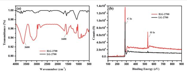
Fig. 6 FTIR spectra (a) and XPS survey spectra (b) of LG-2700 and ILG-2700.
