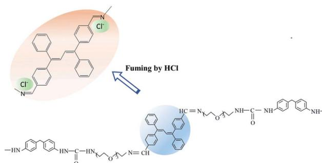
**Fig. 5** The proposed sensing mechanism of the STMPU-50 for the detection of  $\text{HCl}$  gas.
