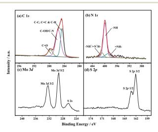
Fig. 1 High-resolution XPS spectra of (a) C 1s, (b) N 1s, (c) Mo 3d, and (d) S 2p of MoS<sub>2</sub>-PANI/rGO nanocomposite.
