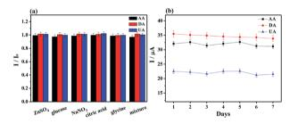
Fig. 7 (a) Peak current ratio of MoS<sub>2</sub>-PANI/rGO/GCE to 1.0 mM AA, 75  $\mu$ M DA, and 75  $\mu$ M UA in the presence of 1 mM of various interfering substances (ZnSO<sub>4</sub>, glucose, NaNO<sub>3</sub>, citric acid, glycine, and the mixture, respectively). (b) The stability of MoS<sub>2</sub>-PANI/rGO/GCE in 0.1 M PBS (pH 7.0, 0.1 M KCI) containing 1.0 mM AA, 75  $\mu$ M DA, and 75  $\mu$ M UA.
