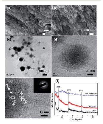
Fig. 2 (a and b) FE-SEM images of MoS<sub>2</sub>-PANI/rGO nanocomposite; (c) TEM and (d and e) HR-TEM images of 3D MoS2-PANI/rGO nanocomposite (the inset in (e) is the corresponding SAED pattern), and (f) XRD patterns of the MoS<sub>2</sub>, MoS<sub>2</sub>/rGO and MoS<sub>2</sub>-PANI/rGO samples.
