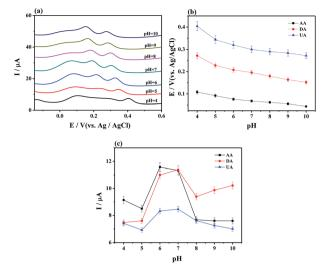
Fig. 4 (a) DPVs of MoS<sub>2</sub>-PANI/rGO/GCE in 0.1 M PBS (pH 7.0, 0.1 M KCl) containing 1.0 mM AA, 75 μM DA, and 75 μM UA with various pH value with in the range from 4.0 to 10.0, and the corresponding peak potential (b) and peak current (c) versus the pH values.
