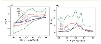
Fig. 3 (a) CV and (b) DPV curves of (i) bare GCE, (ii) MoS<sub>2</sub>/rGO/GCE, (iii) PANI/GCE, and (iv) MoS2-PANI/rGO/GCE in 0.1 M PBS (pH 7.0, 0.1 M KCl) containing 2.0 mM AA, 150 μM DA, and 200 μM UA.
