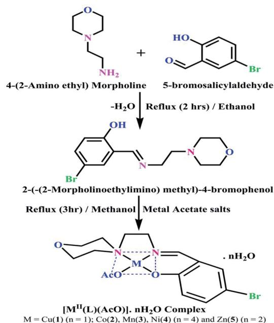
Scheme 1 The proposed structure of complexes 1–5 [M<sup>II</sup>(L) AcO] · nH<sub>2</sub>O.
