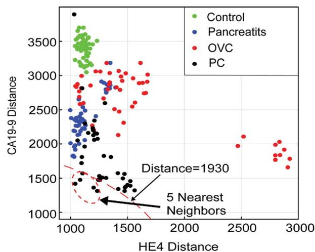
**Fig. 7** Scatter plot of the distance of a sample test data-point from all other data-points in the training set. In this case  $k$  in our K-NN algorithm is set to 5. The point (0,0), which is not shown, is where the test point resides. Looking at the 5-nearest neighbours, one quickly concludes that the test sample should be diagnosed as PC, which in this case is a correct diagnosis.
