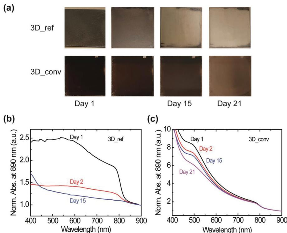
**Fig. 5** Characterization of the moisture stability of the reference and converted 3D FAPbI<sub>3</sub> perovskite films under ambient conditions. (a) Photographs showing the evolution of the color of the reference (top) and converted (bottom) perovskite films over a 21 day period. (b and c) UV-vis absorbance spectra of the reference (b) and the converted (c) films normalized at 890 nm.
