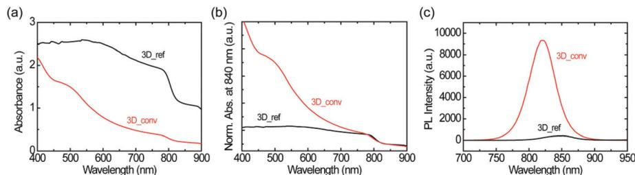
**Fig. 4** Optical characterization of converted and reference 3D perovskite films on glass substrates. (a–b) UV-vis absorbance spectra without normalization (a) and with normalization at 840 nm (b), (c) steady-state PL spectra. Note that 3D\_ref and 3D\_conv as indicated in the figures denote the reference one-step coated and converted FAPbI<sub>3</sub> perovskites, respectively.
