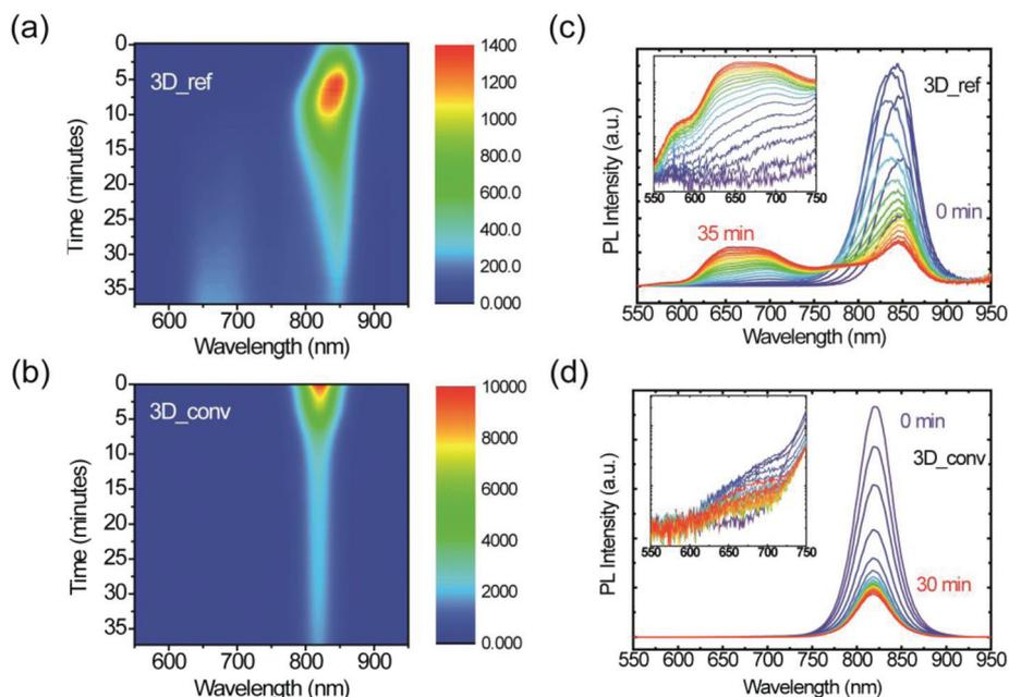
**Fig. 6** Photostability of the reference and converted 3D FAPbI<sub>3</sub> perovskite films. (a) 2D pseudo-color plot of the PL spectra of the reference film as a function of continuous laser excitation time. (b) 2D pseudo-color plot of the PL spectra of the converted film as a function of continuous laser excitation time. (c) Evolution of the PL spectra of the reference film. (d) Evolution of the PL spectra of the converted film.
