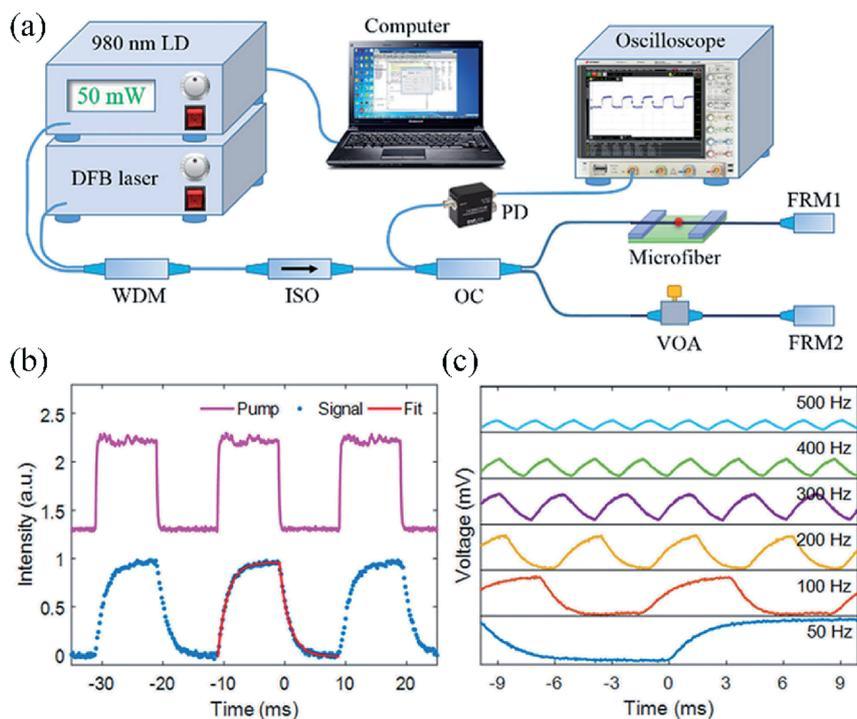
Fig. 5 (a) A MI fiber all-optical modulator based on bismuthene material. (b) Waveforms of control light (pump) and signal light and the corresponding fitting curve. (c) Signal waveforms at different modulation frequencies of control light (pump). This figure has been adapted from ref. 12 with permission from *Journal of Materials Chemistry C*.
