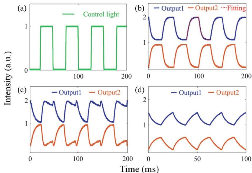
Fig. 4 (a) Waveform of the control light (pump). (b) A single on–off transition of the signal light and the corresponding fitting curve. (c) Output breaking. (d) Waveforms of signal light at 40 Hz. This figure has been adapted from ref. 16 with permission from *Advanced Materials*.
