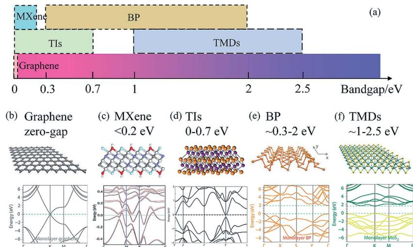
**Fig. 1** (a) Distribution diagram of the bandgap of 2D materials. The atomic structures and band structures (monolayer) of graphene, (b) MXene, (c) TIs, (d) BP (e) and TMDs (f). This figure has been adapted from ref. 37, 61, 69 and 76 with permission from *Nature Physics*, *Advanced Materials*, *Nature Photonics*, *Journal of the American Chemical Society*.
