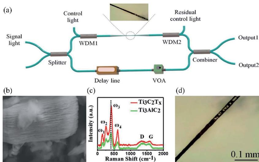
Fig. 2 (a) Experimental setup of an MZI all-optical modulator based on MXene materials. (b) High-resolution electron microscopy image of MXene nanosheets. (c) Raman spectrum of  $\text{Ti}_3\text{AlC}_2$  and  $\text{Ti}_3\text{C}_2\text{T}_x$ . (d) Optical microscopy image of microfibers deposited with MXenes. This figure has been adapted from ref. 16 with permission from *Advanced Materials*.
