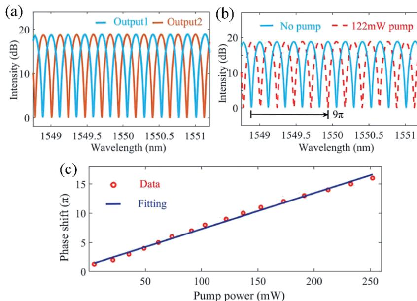
Fig. 3 (a) Interference spectra of two output ports. (b) Interference fringes at a control light (pump) power of 122 mW. (c) Phase shift versus different control light (pump) powers. This figure has been adapted from ref. 16 with permission from *Advanced Materials*.
