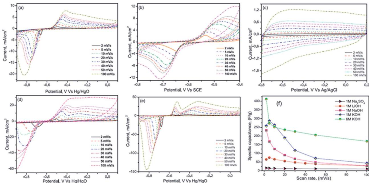
Fig. 9 CV curves at various scan rates of (a) 1 M LiOH (b) 1 M NaOH (c) 1 M Na<sub>2</sub>SO<sub>4</sub> (d) 1 M KOH and (e) 6 M KOH and (f) capacitance vs. scan rate for different electrolytes. This figure has been adapted from ref. 116 with permission from Elsevier.
