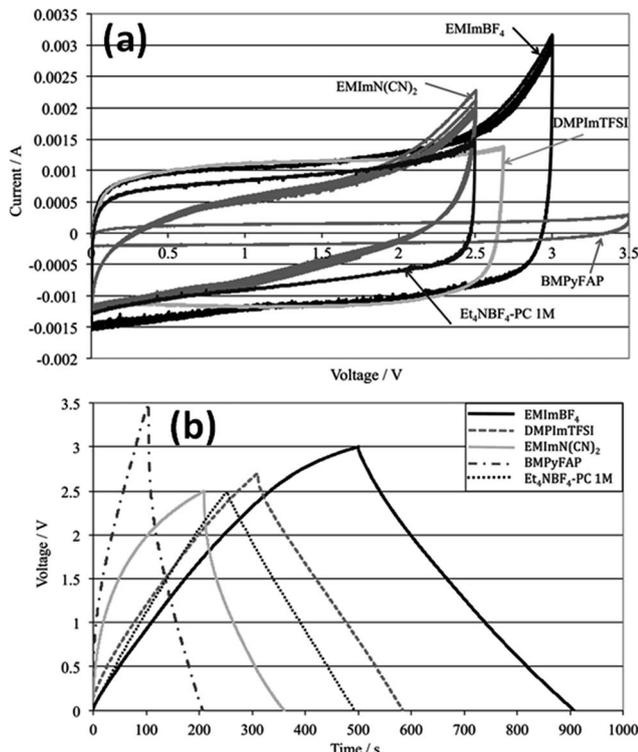
Fig. 18 (a) CV of various electrolytes at  $5 \text{ mV s}^{-1}$  and (b) galvanostatic charge-discharge at  $2 \text{ mA cm}^{-2}$ . This figure has been adapted from ref. 168 with permission from the Royal Society of Chemistry.
