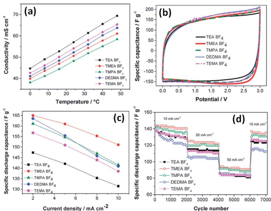
Fig. 13 (a) Conductivity values vs. temperature, (b) CV in various electrolytes at  $2 \text{ mV s}^{-1}$ , (c) capacitance values at low currents, and (d) cycle life tests. This figure has been adapted from ref. 121 with permission from the Royal Society of Chemistry.
