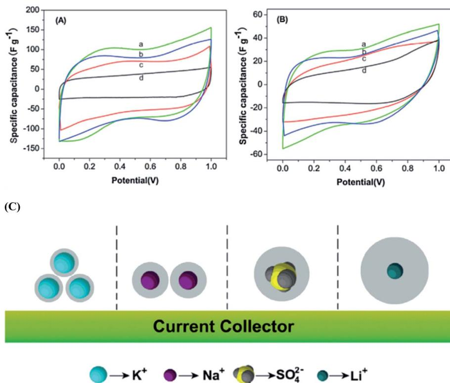
Fig. 10 CV curves of the supercapacitors with the electrolytes (2 M) (a) KOH, (b) NaOH, (c) LiOH and (d)  $\text{Na}_2\text{SO}_4$  at scan rates of (A)  $5 \text{ mV s}^{-1}$  and (B)  $100 \text{ mV s}^{-1}$ . (C) The ion of hydrated ionic radius on the  $\text{MnFe}_2\text{O}_4$ -based supercapacitors. This figure has been adapted from ref. 117 with permission from Elsevier.
