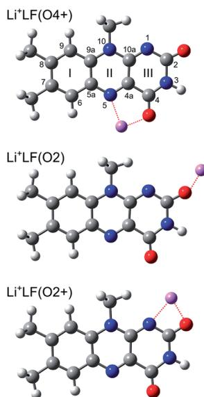
Fig. 1 Structures of relevant M<sup>+</sup>LF isomers calculated at the PBE0/cc-pVDZ level of theory illustrated for M = Li, along with atom and ring numbering. N/O atoms are indicated in blue/red colour.
