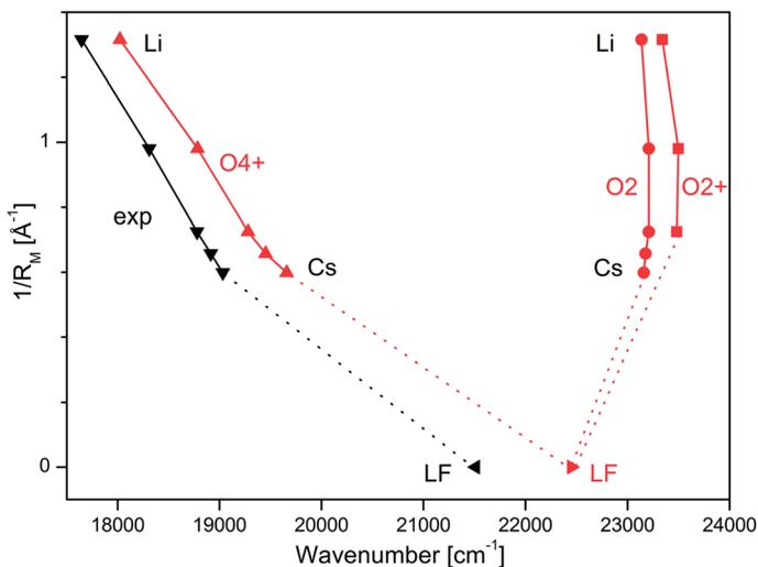
Fig. 3 Experimental  $S_1$  origins extracted from the VISPD spectra of  $M^+LF$  compared to adiabatic  $S_1$  origin energies of the O4+ and O2(+) isomers of  $M^+LF$  calculated at the PBE0/cc-pVDZ level plotted as a function of the inverse ionic radius of the metal ion ( $1/R_M$ ). The  $M^+LF$  ions with  $M = Rb$  and  $Cs$  do not have a stable O2+ structure. The experimental value for LF is taken from the He droplet spectrum.<sup>55</sup>
