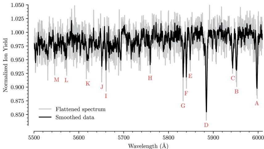
Fig. 1 Absorption spectrum in a range from 5500 Å to 6000 Å of  $C_{20}H_{10}^+$  complexed with a single He atom. The flattened raw spectrum is shown in gray and is overlaid with a spectrum where the data has been smoothed (moving average over 10 nearest neighbors) for easier viewing. All of the analysis is performed on the unsmoothed dataset. Identified absorption lines are labeled and their positions are reported in Table 1.
