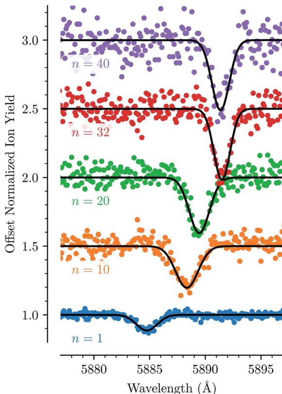
Fig. 2 The absorption feature of  $\text{He}_n\text{C}_{20}\text{H}_{10}^+$  near 5885 Å (line D) shown for different numbers of  $n$ . The line is redshifted in a non-linear fashion up to  $n = 32$ , after which the position is very slightly blue-shifted again. Gaussian fits are shown as solid black lines.
