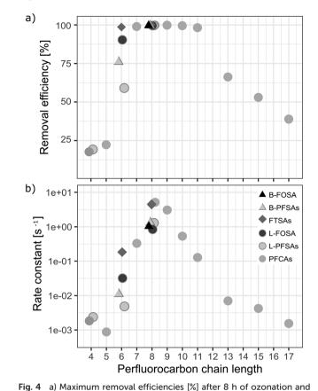
b) second order reaction rate constants [s<sup>-1</sup>] for all analyzed PFASs of varying perfluorocarbon chain lengths and functional groups in the pilot-scale ozonation treatment. Rate constants were calculated according to the second order rate law described by Atkins et al. 50
