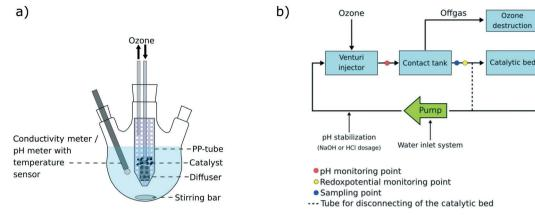
Fig. 1 a) Experimental set up of the 500 mL laboratory-scale system and b) scheme of the 50 L pilot-scale system.
