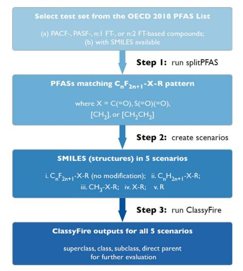
Fig. 2 Step-by-step workflow for selecting, splitting, modifying and categorizing PFASs in the current work
